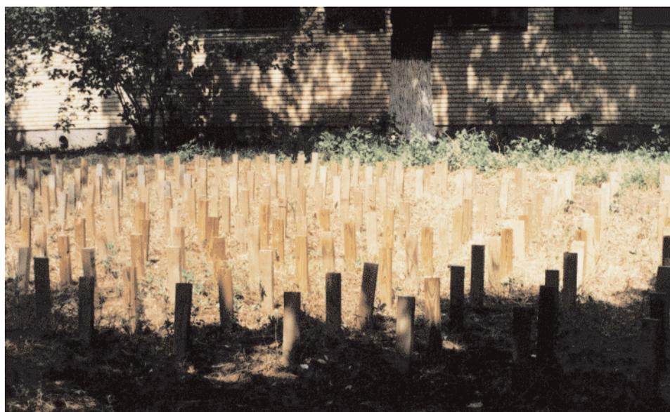
**Figure 1.** Field test. Samples treated with CCA type product exposed in the test site
